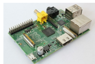
Fig. 2: A view of a Raspberry Pi 1 board.
